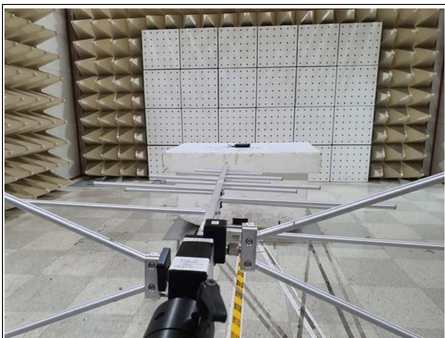
**3. Photo of Radiated Spurious Emission Test (Above 1 GHz)**
