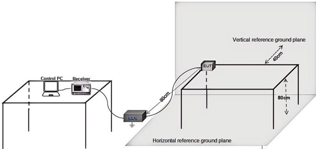
Description of test setup connection:
