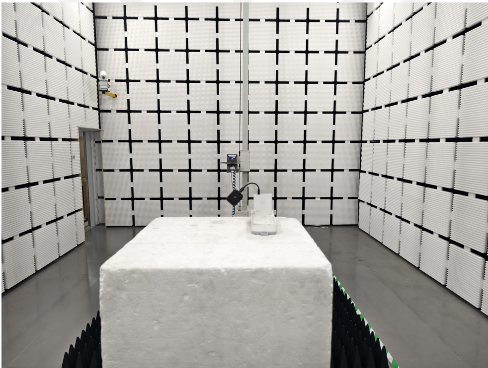
Spurious Radiation Emissions Test (> 1G)
