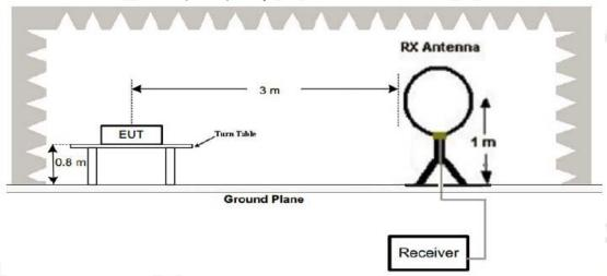
2. Radiated Emission Test-Up Frequency 30MHz~1GHz
