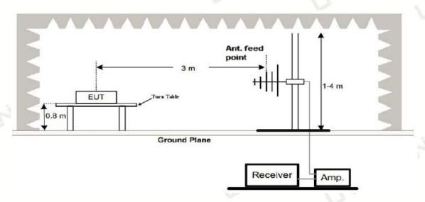
3. Radiated Emission Test-Up Frequency Above 1GHz
