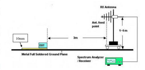
**Below 1000MHz Test Setup**
