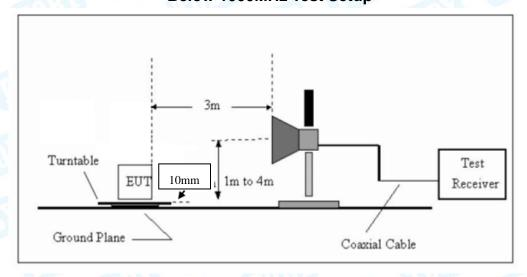
**Above 1GHz Test Setup**
