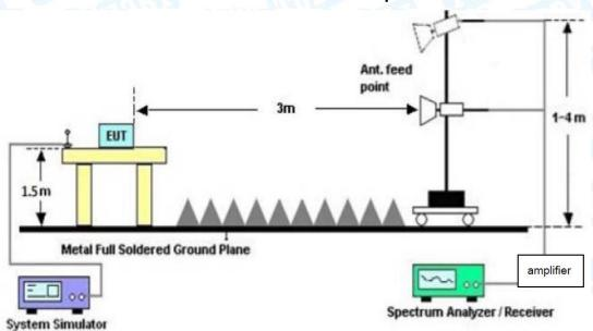
**Above 1GHz Test Setup**
