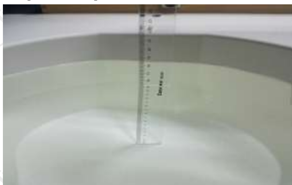
The Body Liquid of 2450MHz (15.3cm)
