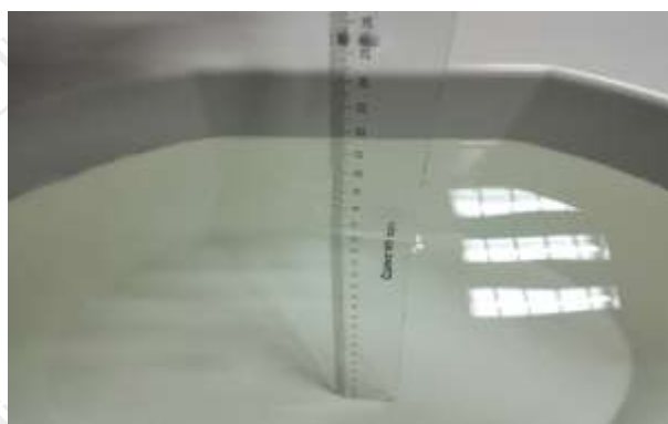
The Body Liquid of 5000-6000MHz (16.5cm)
