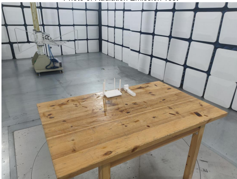
Photo of Radiation Emission Test
